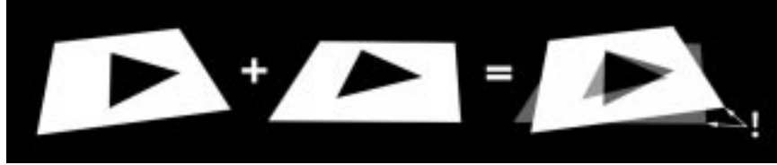
Figure 1.1: Unregistered projections. If shadow projections are done with a standard perspective camera then views from different light samples do not line up.
